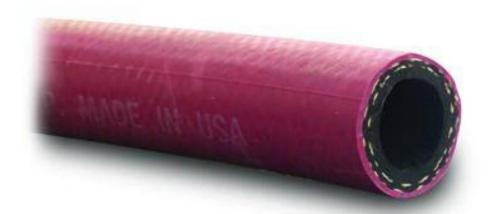
Multipurpose is an EPDM hose designed for continuous flow hose reels. It's our toughest and most durable non-collapsible hose. The EPDM tube and cover, reinforced with polyester yarn allows Mutlipurpose to be used in a variety of environments as well as remain fully functional in cold temperatures. Suitable for fire protection or industrial applications. Available in a variety of lengths and sizes (see below).
